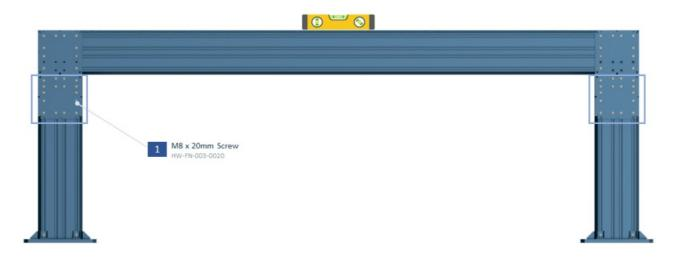
10. Now it's time to install the leveling mechanism. First, install the ST-SP-016-0003 on Assembly Plate with 2x M8x20 mm like in the picture below.
