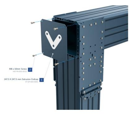
Note: Use High Strength Thread Locker (HW-CS-001-0003) to prevent the screws from loosening over time due to vibration.
