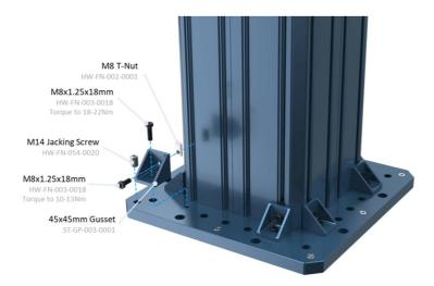
3. Check if the above assembly is perpendicular to the floor using a level by Placing it on 2 sides of the column. If the column is not level, use 8x M14 set screws (HW-FN-054-0020) on the plate to level it.
