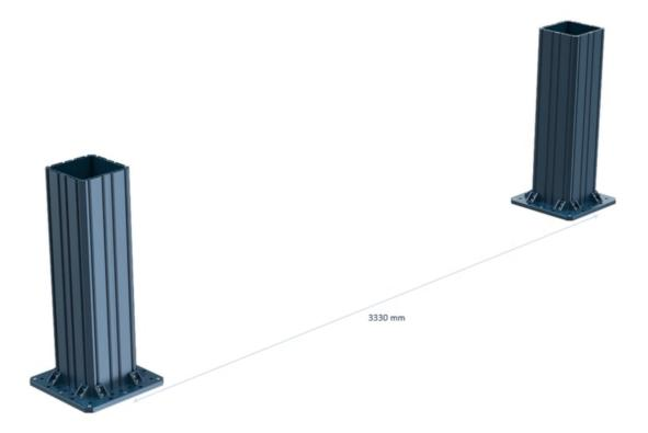
6. Place the 3330 mm horizontal beam on top of these 2 columns. For lifting the beam, you can use one of the methods explained in the **Recommended** Handling Methods section at the bottom of this page.
