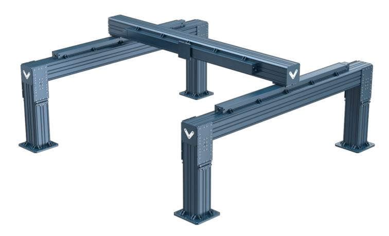
Note: Special attention must be given to the alignment of the parallel structures. Use of high precision bearing systems rigidly mounted in a parallel configuration requires horizontal positional tolerances of 0.025mm or 0.001". Height tolerances are also important but are much less tight. For additional information on alignment requirements reach out to our Application Engineering team.
