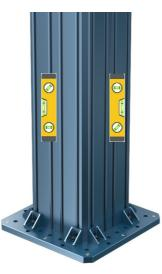
4. Once the column is level and in the correct location, use the shim kit (<u>HW-SH-001-0001</u>) to fill the gap between the plate and the floor. Install the shims and anchor bolts in the shown location according to the picture below. The shim slot should hug the anchor bolt. Use 8x 1/2 inch anchor bolts from the anchoring kit (<u>ST-RB-033-0002</u>) to anchor the plate to the floor. The holes can be drilled in concrete using a hammer drill.
