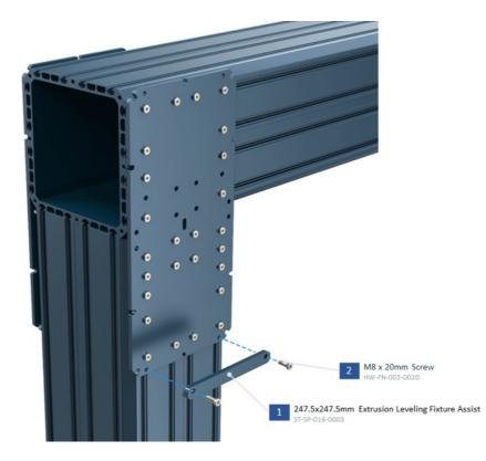
11. Install **ST-SP-016-0002** by tightening the shown **6x M8x20 mm** screws. Then using **2x M10x40 mm** you can move the assembly plate up and down and level the horizontal beam. Install one leveling mechanism for each assembly plate on both sides of the column.
