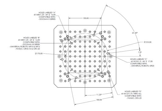
Note: \* The mounting angle of the CRX-25 is clocked at 11.25 degrees. The UR20e is also clocked at 7.5 degrees. If you would like to mount these robots orthogonally, see the supported robot plate below.
