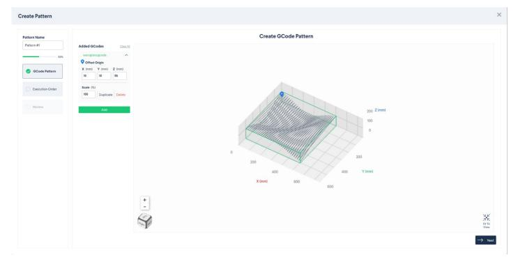
You can use the X, Y, and Z inputs to translate the file in 3D space:
