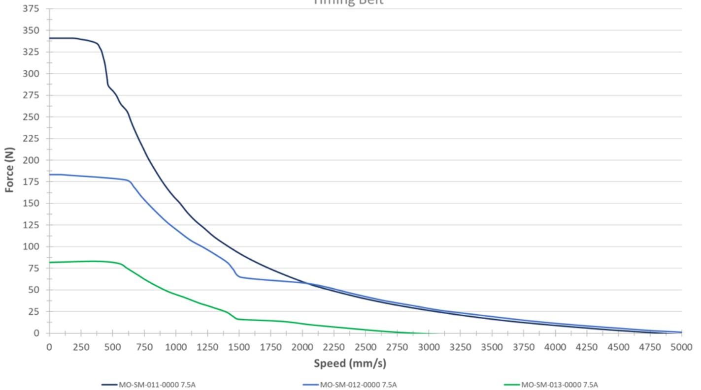
Observing the figure above, the force slowly decreases as the linear velocity increases, making the timing belt actuator ideal for lower force applications that require higher movement speeds. If more force is required and travel speed is not as critical, consider adding a gearbox to the powertrain. See the below figure for expected performance with a gearbox.
