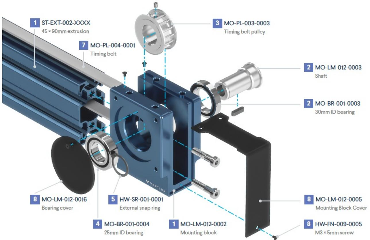
1. Tap the end of the extrusion and mount the end block using 2 X M8 X 35mm screws.
