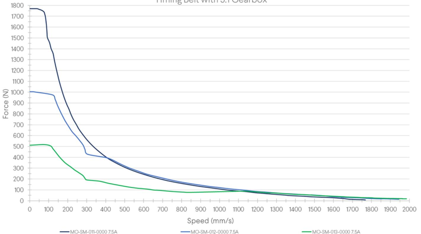
Observing the figure above, the force is much higher when using the gearbox, however it decreases much faster as the linear velocity increases. This makes the combination ideal for slower moving applications with higher forces.
